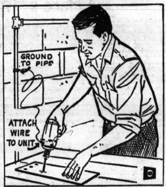
SAFETY FIRST —Power tool properly grounded is the best health insurance you can have in the workshop. If unit is not equipped, run ground wire from convenient screw or bolt to heating or plumbing pipe.
