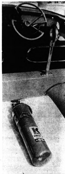
SAFETY DEVICE — Motorboats are required to be equipped with fire extinguishers. Larger boats require more than one extinguisher.
