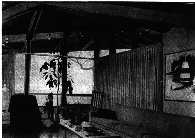
Overhang Is Designed To Let Sun In During Wintertime And 'Keep It Out In Summer
