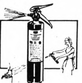
Dry Chemical Fire Extinguisher
