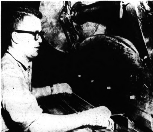
BENDER — A power brake bends pieces of aluminum for angle front wheelhouse supports. Leo Hess, 44 Prall St., says he and the machine can turn out 500 pieces an hour.
