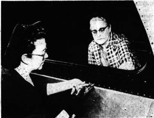
RIVETERS — It takes two people to rivet panels in place on the back end of this bus. Mrs. Vida Wagner, 154 Edison St., applies the riveter while Mrs. Ida Williams, 216 Central St., holds the "bucking bar" in place to absorb the shock.
