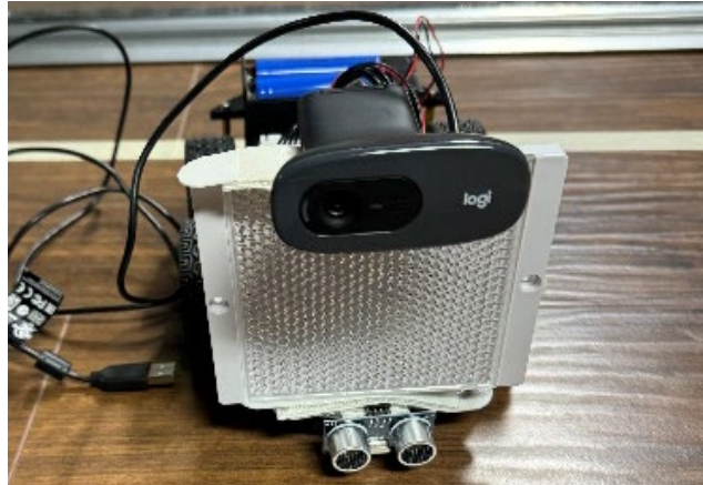
Figure 5.13 Webcam mounted to the rear car captures the front car
