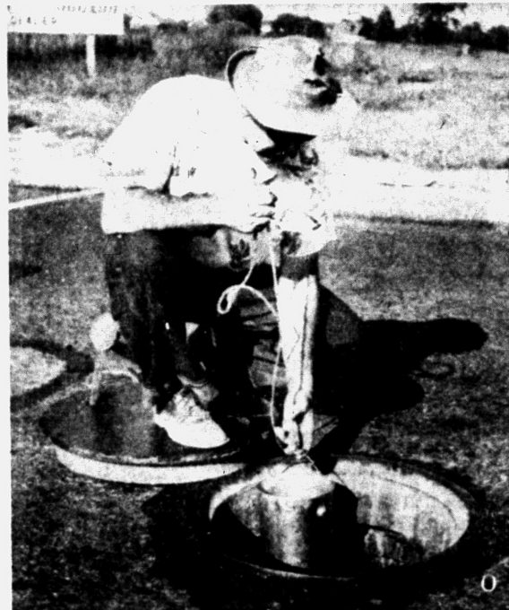
HUNT WATER POISON — Oliver Prudhomme, DPW employee, dips up a sample of sewer water at East Blvd. and South Blvd. as the search for the source of the chromium wastes contaminating the Clinton River continues. Gordon E. Olivier, sanitary engineer for the
