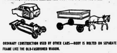
IN JET AIRCRAFT, STRUCTURAL MEMBERS AND FUSELAGE ARE ONE AND THE SAME. IN RAMBLER, STRUCTURAL MEMBERS AND BODY ARE ONE AND THE SAME.
