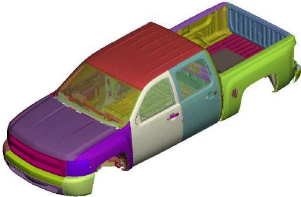
Figure 6.10 Finite element model of Silverado pickup truck
