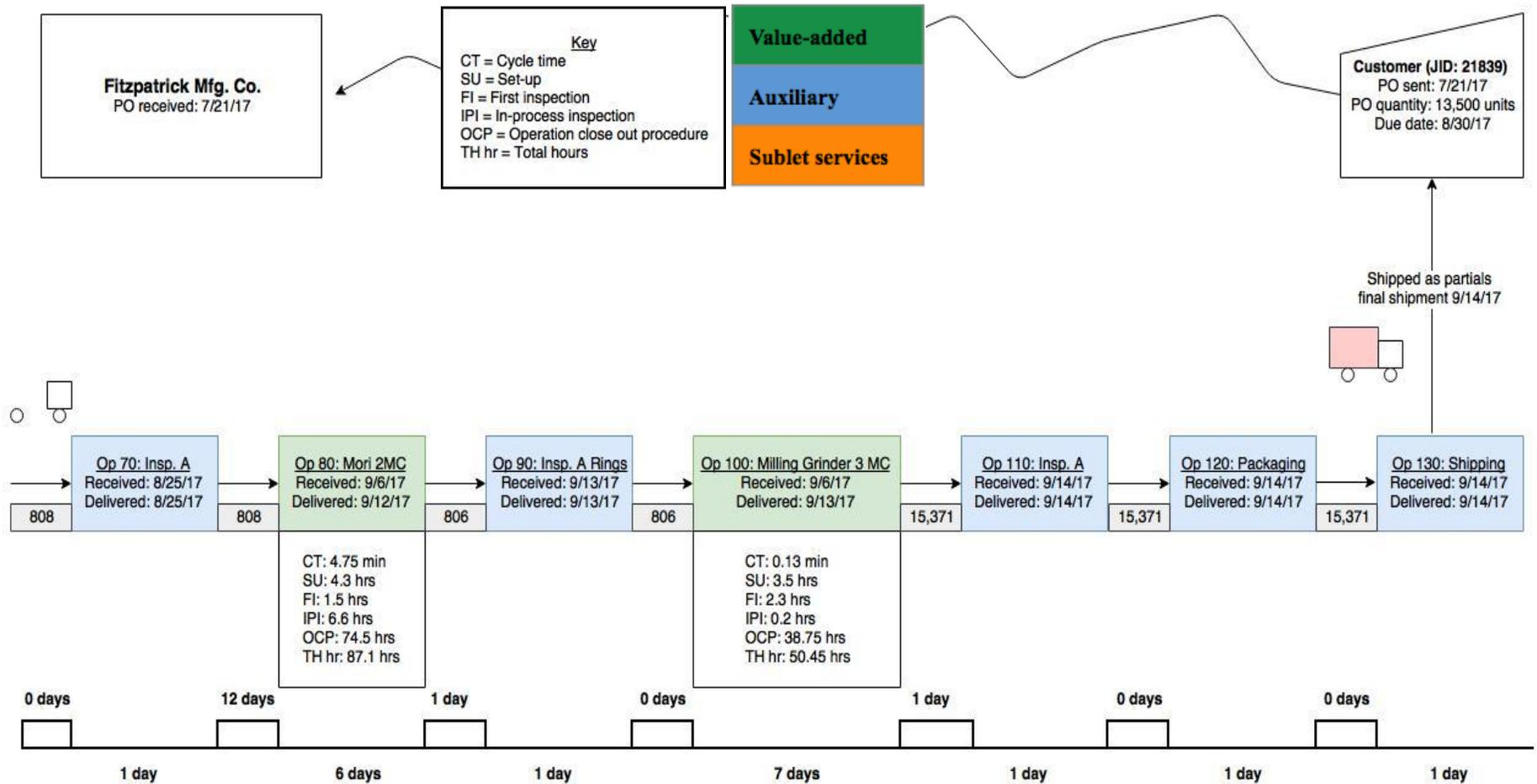
Figure 4: Current condition of FMC's sublet shipping process
