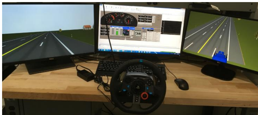
Figure 5.3. The hardware-in-the-loop bench setup with the steering wheel to manually drive the ego vehicle on real time basis.
